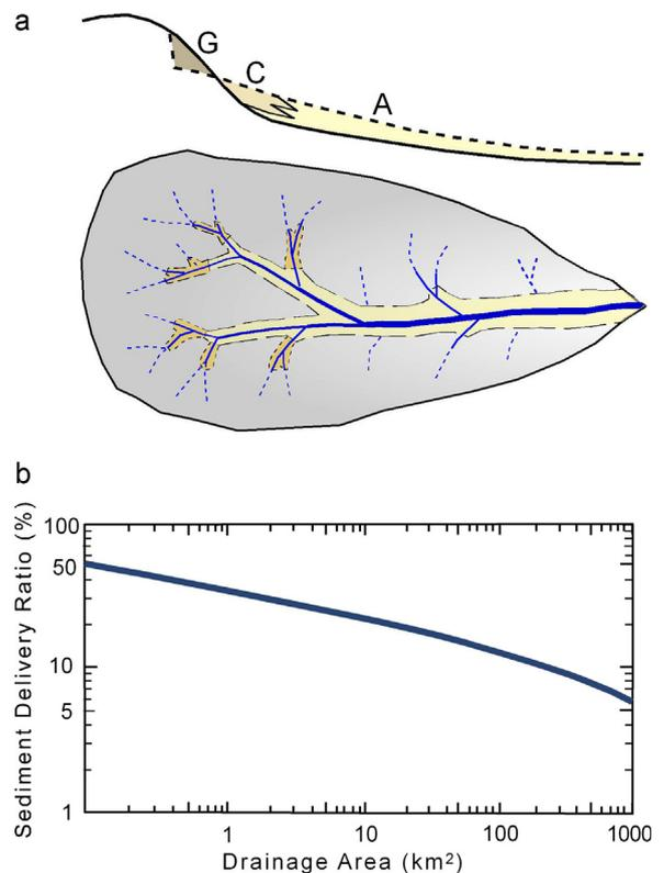
**Fig. 8.** Downstream changes in sediment deliveries due to storage in bed (A) result in rapidly decreasing sediment delivery ratios downstream (B). G: gully; C: colluvium; A: alluvium.
