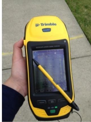
Figure 4: GPS Unit-TrimbleGeoXT 6000
