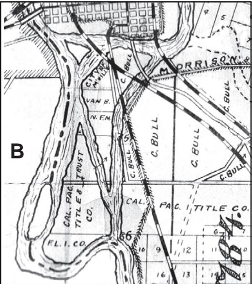
Figure 12. Channelization around Yuba-Feather confluence. Several ditches were dredged south of Marysville shortly before 1909. Two ditches connected with the Feather River at Elisa Bend, and another turned the confluence south. (A) Stratigraphic sections collected at XS are shown in Figures 13 and 15A. (Source: CDC, 1912.) (B) Ditches are prominent (cartographically exaggerated) on 1914 map. (Source: Crook, 1914.)
