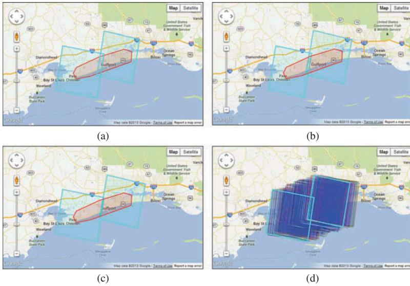
Figure 8. Top three image collection plans derived from the optimization model, (a), (b) and (c) represents #1, #2 and #3 solution in Figure 7, respectively. (d) shows the spatial coverage of the first solution over 169 available image collection opportunities.
